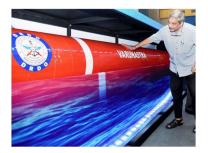
Varunastra is a ship-launched, electrically-propelled underwater weapon equipped with one of the most advanced automatic and remote-controlled guidance systems. The weapon system uses its intelligence in tracing the target. It can hit stealth submarines underwater.
